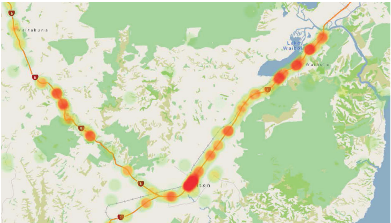
Heat Map of high risk accident spots 2013-2018. Scale from yellow to red (red indicating highest volume of serious or fatal crash sites)
