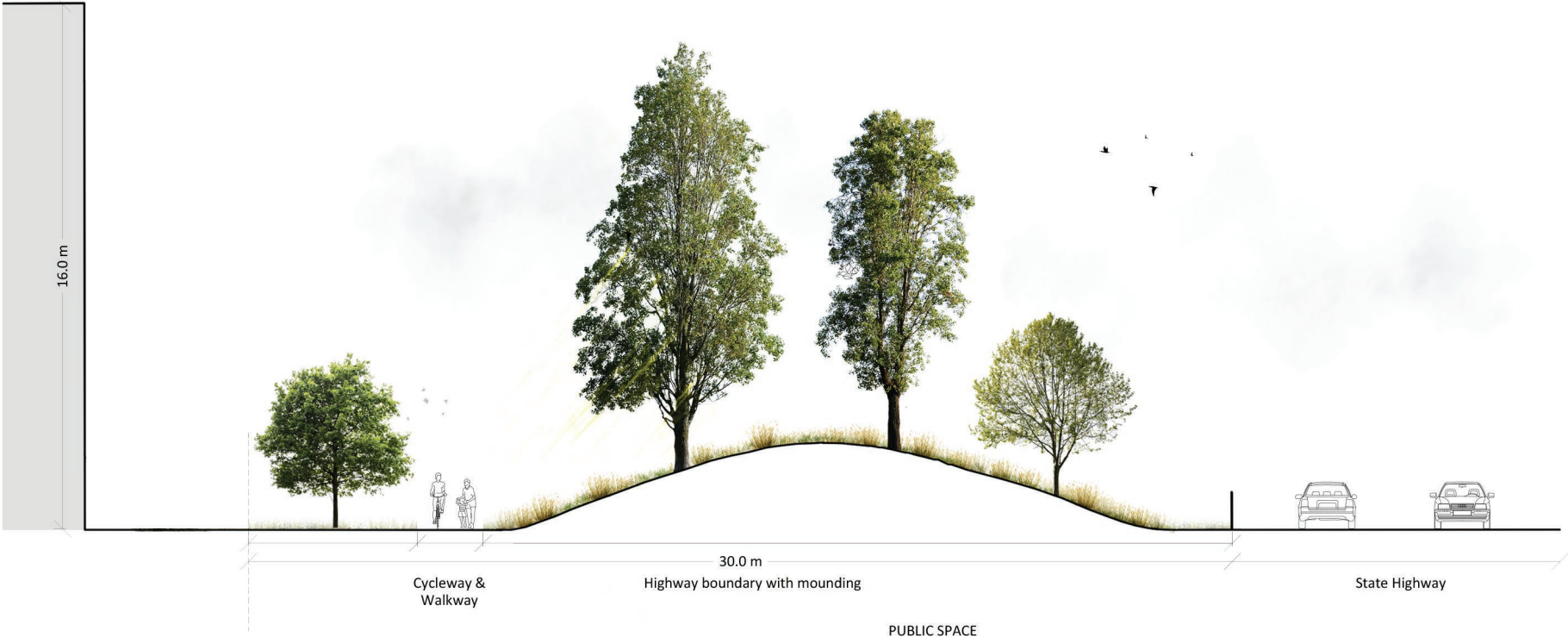
Figure 10 : 30m Highway Boundary (mounding)
