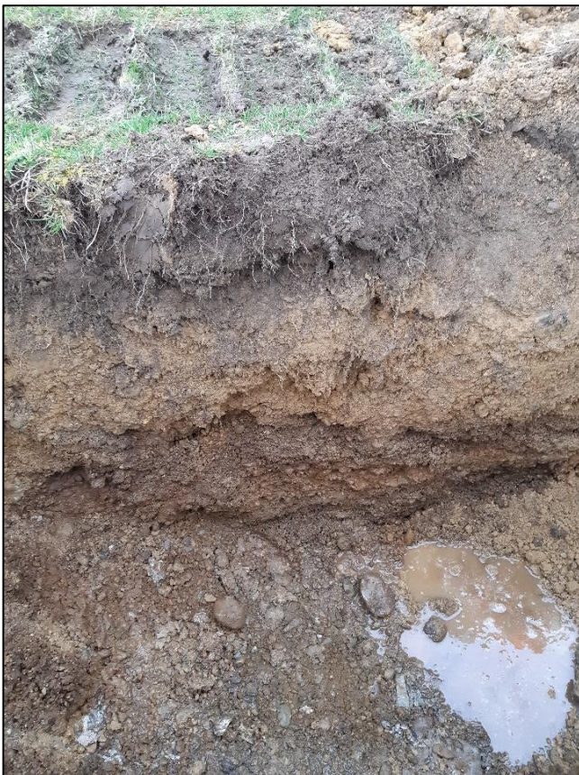
Figure 18. General strata throughout the geotechnical trial pits
