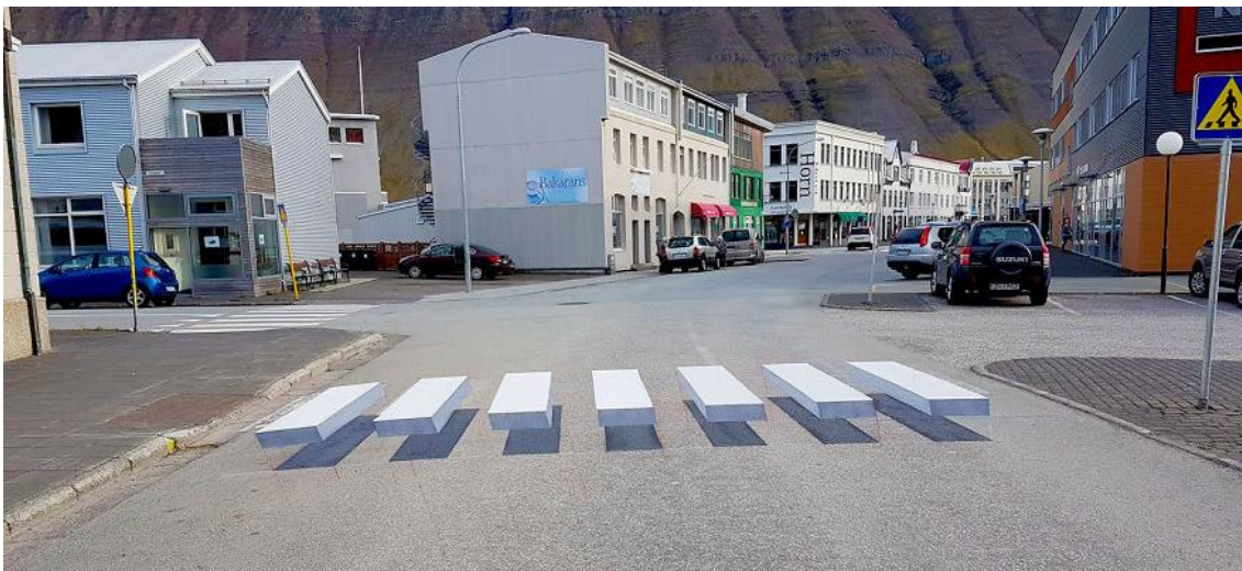
Figure 9. A painted road crossing, using a 3-D design, to give the appearance of rising above the road, to help slow traffic as it enters a town in Iceland. 3
