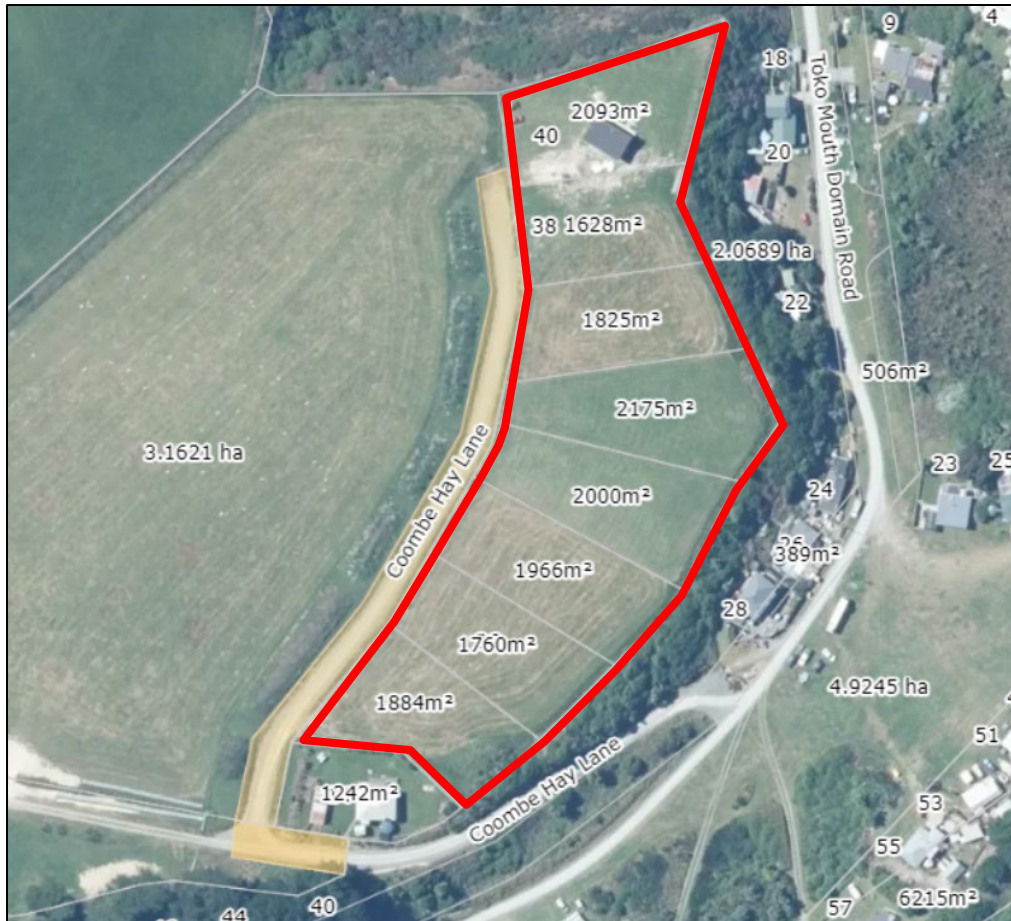
Figure 5: Aerial photograph illustrating the previous subdivision which created eight residential allotments (red outline) and the Coombe Hay Lane ROW, identified by the two areas with yellow shading (Source: Gripp Survey App). The eastern original portion of Coombe Hay Lane is located on Road.
