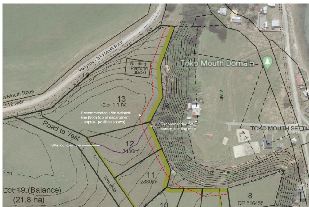
Figure 8: Excerpt of Figure 1 from the Landscape and Natural Character Assessment. The plan shows the 15m setback from the escarpment (red dashed line) and the 96m contour (purple line).
