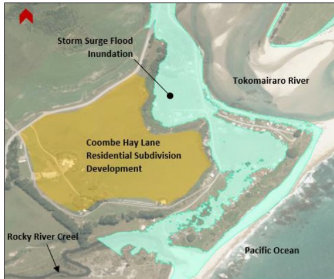
Figure 2.1: Storm Surge Inundating Low-lying Areas Downstream to Site
