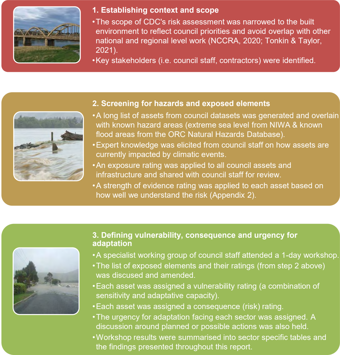
Figure 2-1 Diagram showing the climate change risk methodology process, adapted from the NCCRA guidelines
