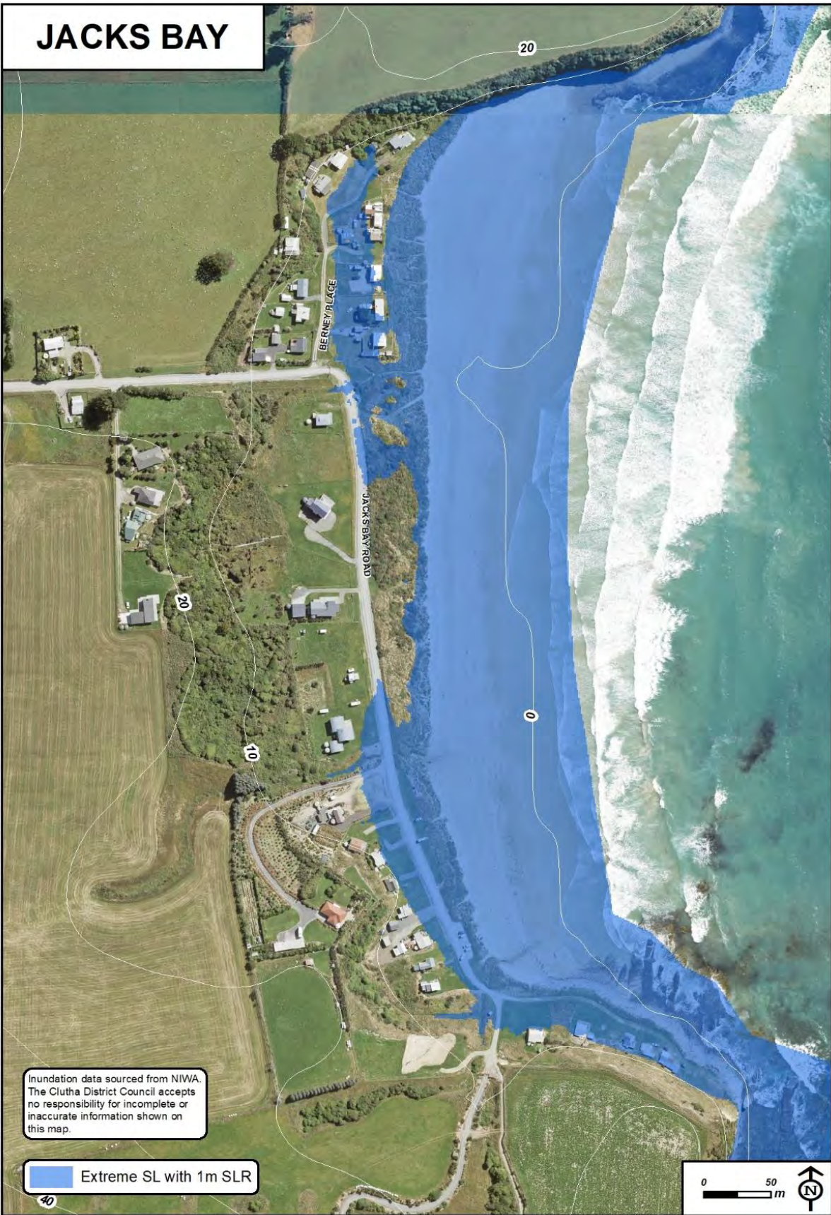
Figure 4-12 Land which is potentially exposed to coastal inundation at Jacks Bay (shaded blue), during a 1:100-year extreme sea level event, together with 100 cm of sea level rise. Smaller increments of sea level rise may also have an impact on this settlement, and a 50 cm SLR scenario is shown in Appendix 2.
