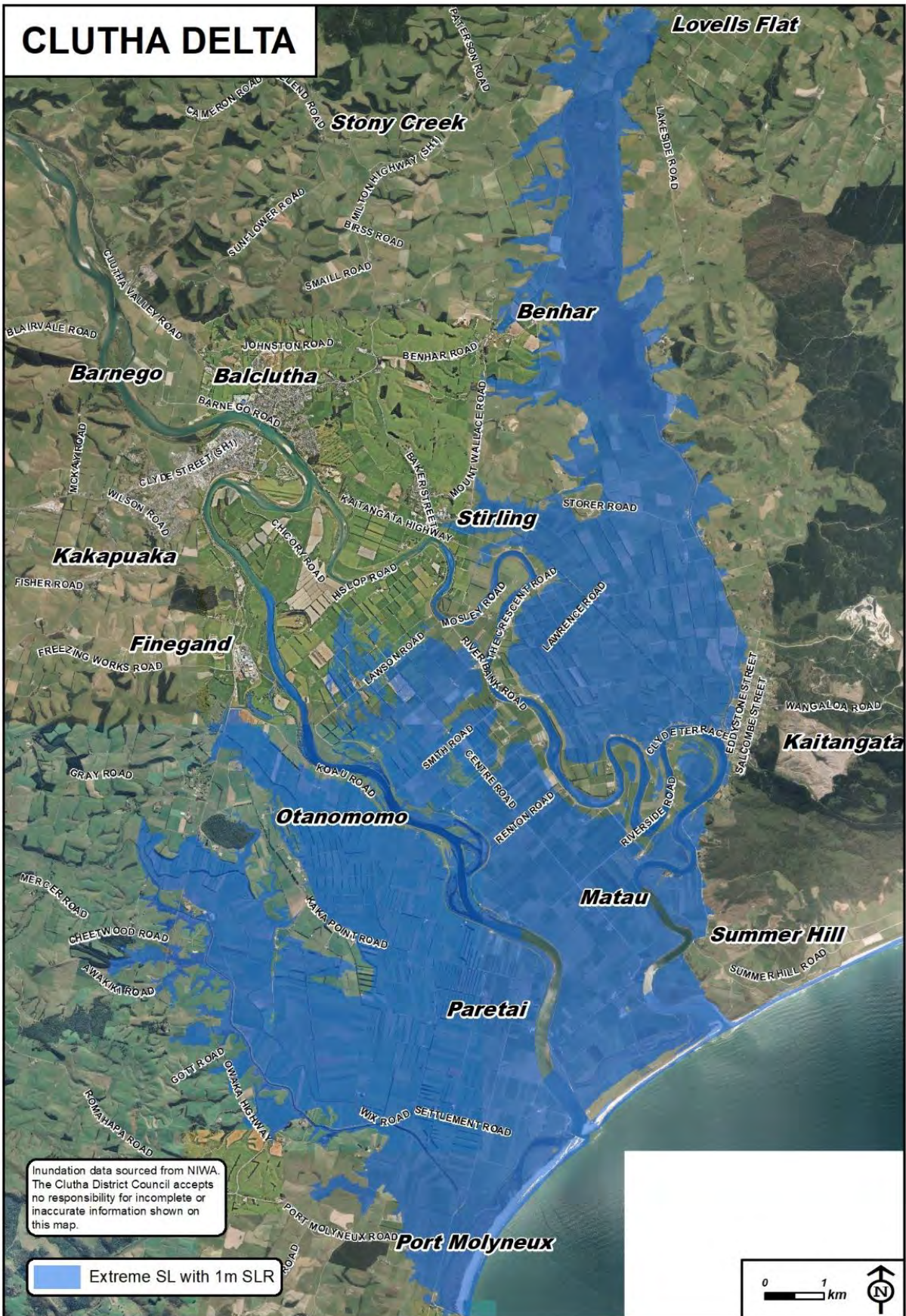
Figure 3-12 Land which is potentially exposed to coastal inundation on the Clutha Delta (shaded blue), during a 1:100-year extreme sea level event, together with 100 cm of sea level rise. Smaller increments of sea level rise may also have an impact on this area, and a 50 cm SLR scenario is shown in Appendix 2.
