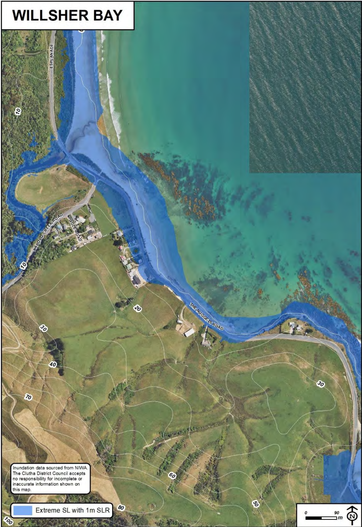
Figure 4-9 Land which is potentially exposed to coastal inundation at Willsher Bay (shaded blue), during a 1:100-year extreme sea level event, together with 100 cm of sea level rise. Smaller increments of sea level rise may also have an impact on this area, and a 50 cm SLR scenario is shown in Appendix 2.
