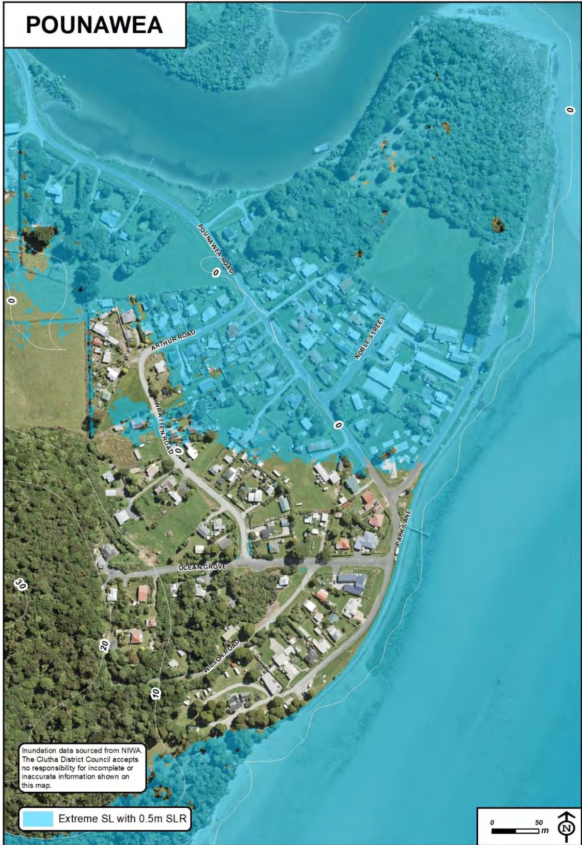
Figure A2.9 Land which is potentially exposed to coastal inundation at Pounaweia (shaded blue), during a 1:100-year extreme sea level event, together with 50 cm of sea level rise.
