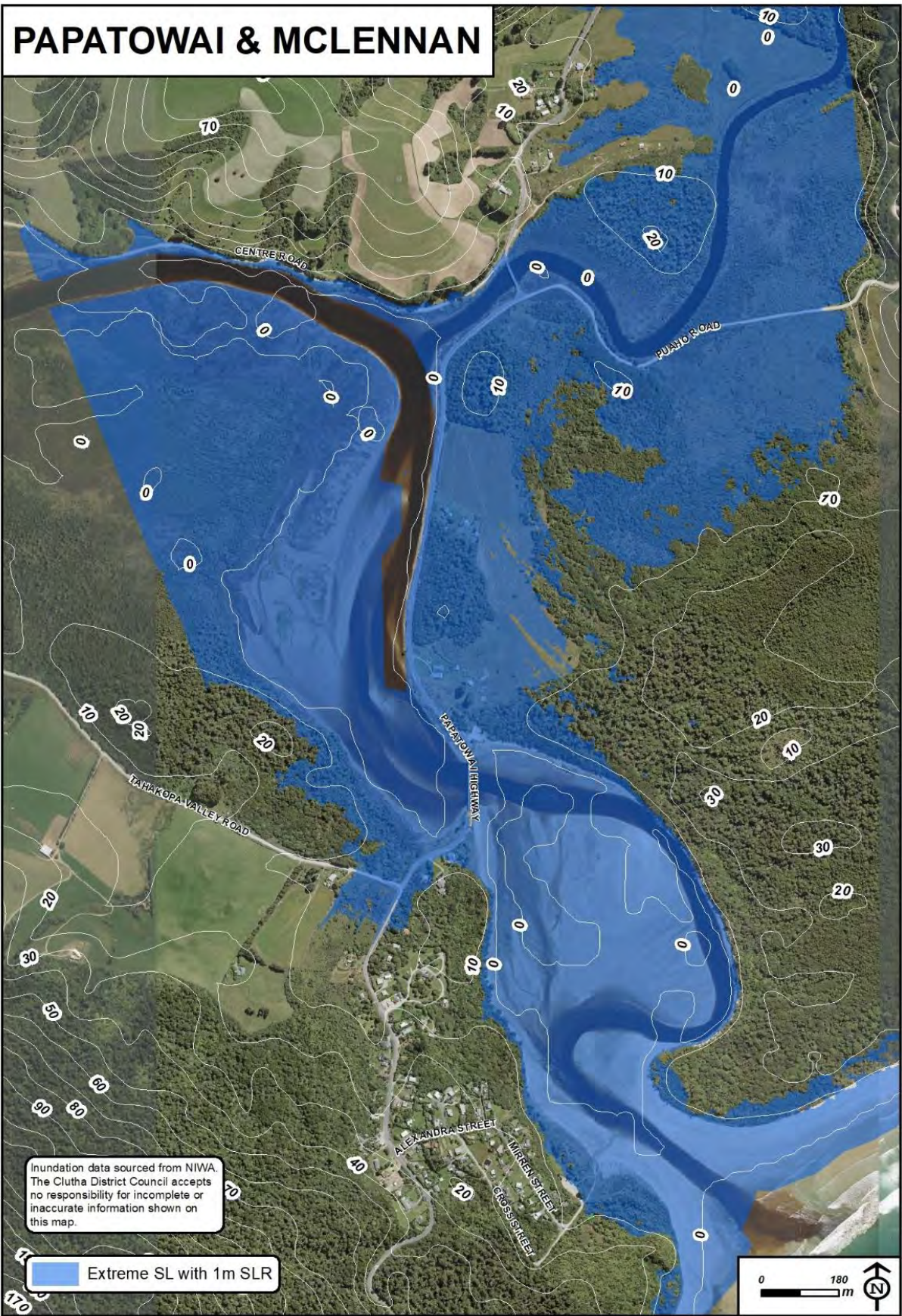
Figure 4-13 Land which is potentially exposed to coastal inundation at Papatowai and MacleNNAN (shaded blue), during a 1:100-year extreme sea level event, together with 100 cm of sea level rise. Smaller increments of sea level rise may also have an impact on this area, and a 50 cm SLR scenario is shown in Appendix 2.
