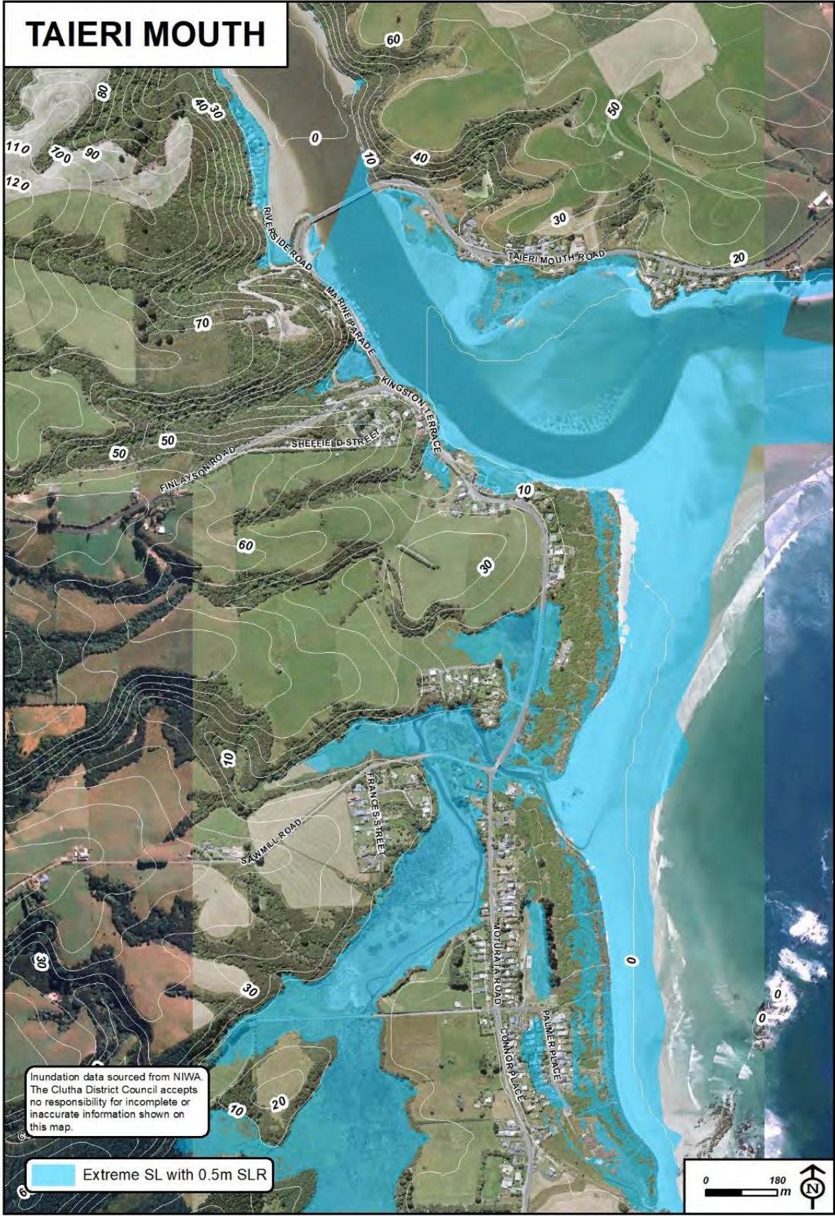
Figure A2.1 Land which is potentially exposed to coastal inundation at Taieri Mouth (shaded blue), during a 1:100-year extreme sea level event, together with 50 cm of sea level rise.
