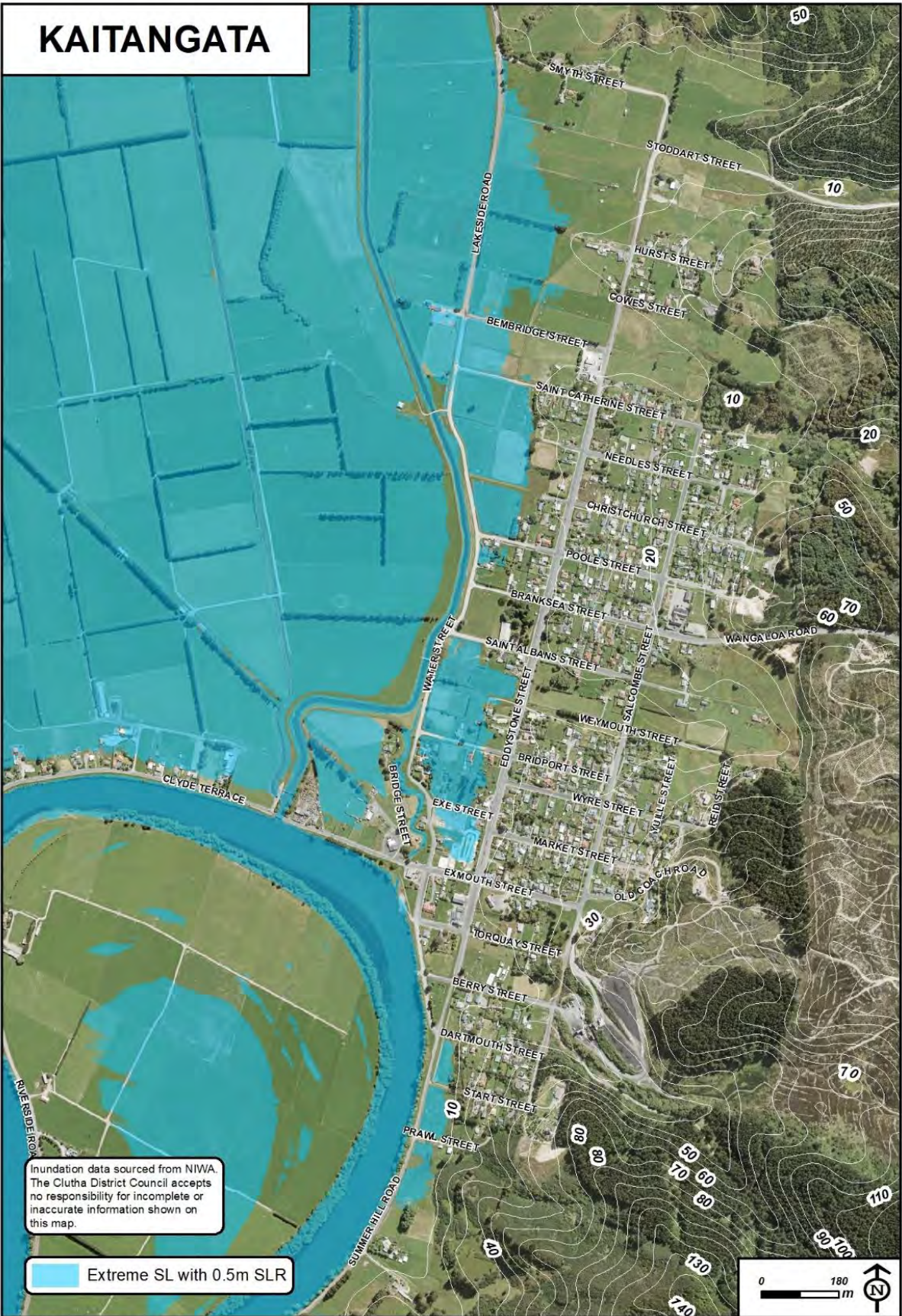
Figure A2.5 Land which is potentially exposed to coastal inundation at Kaitangata (shaded blue), during a 1:100-year extreme sea level event, together with 50 cm of sea level rise.
