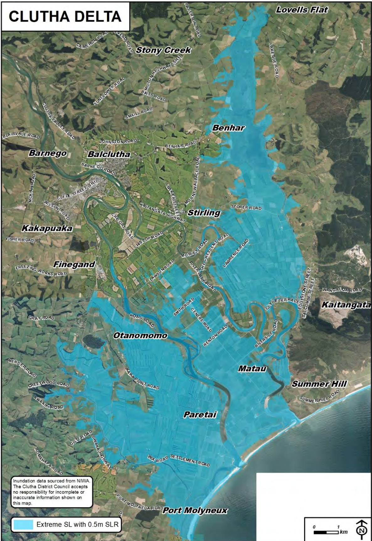
Figure A2.6 Land which is potentially exposed to coastal inundation on the Clutha Delta (shaded blue), during a 1:100-year extreme sea level event, together with 50 cm of sea level rise.
