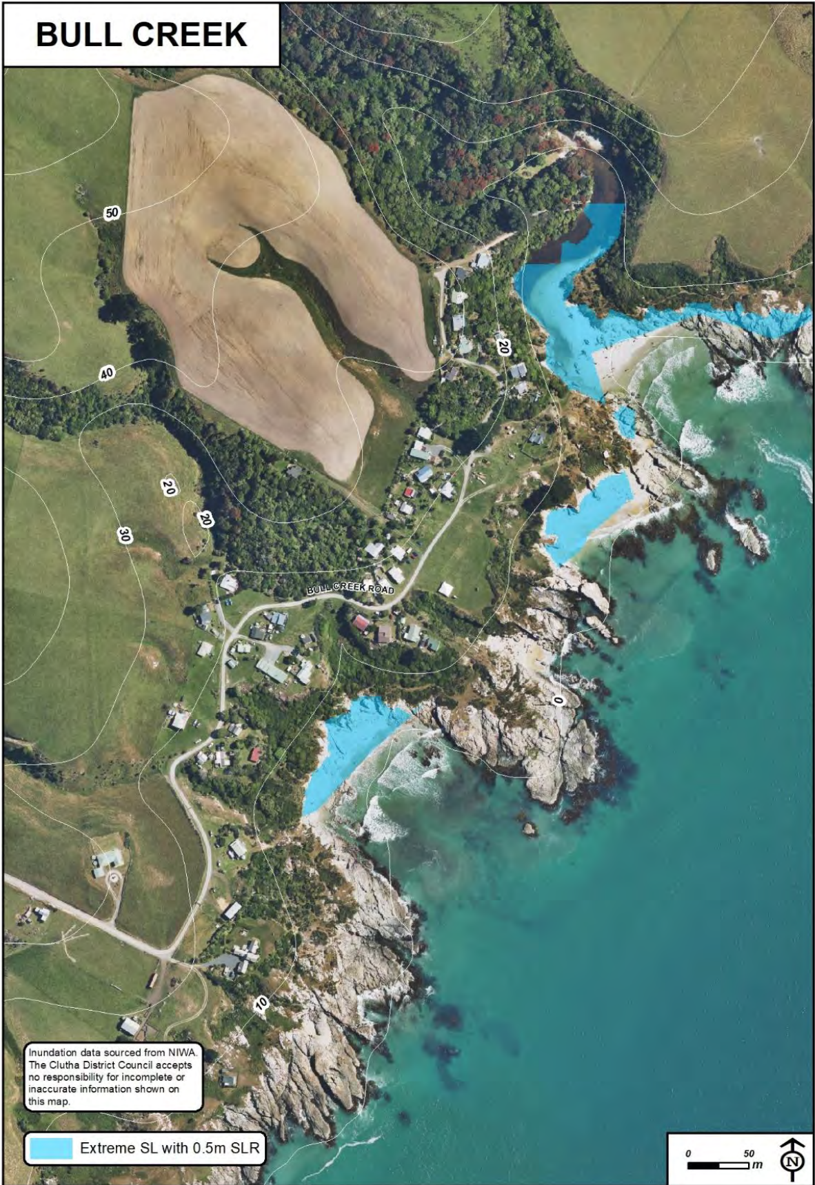
Figure A2.3 Land which is potentially exposed to coastal inundation at Bull Creek (shaded blue), during a 1:100-year extreme sea level event, together with 50 cm of sea level rise.
