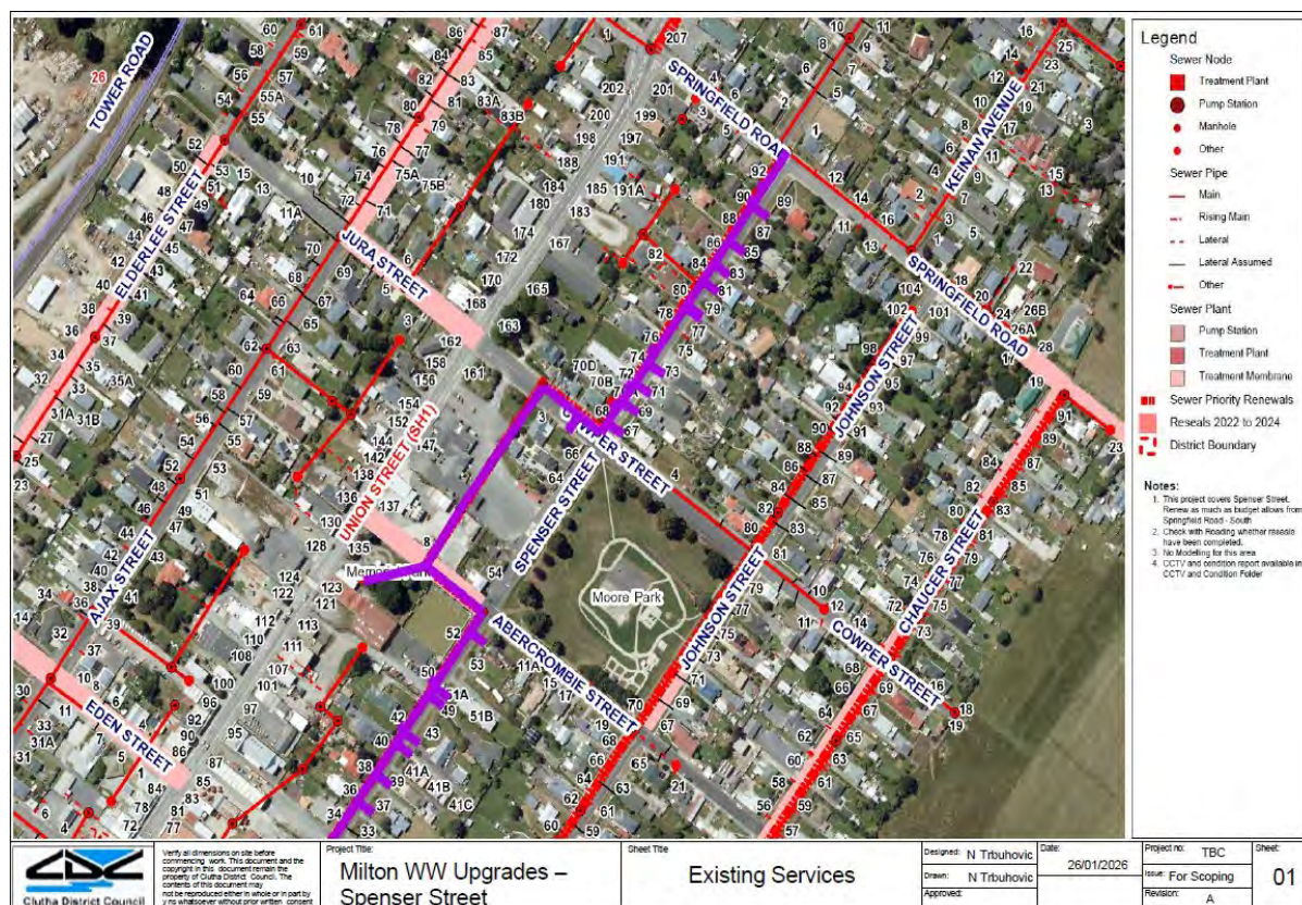
Figure 1: Spencer Street sewer network renewal
