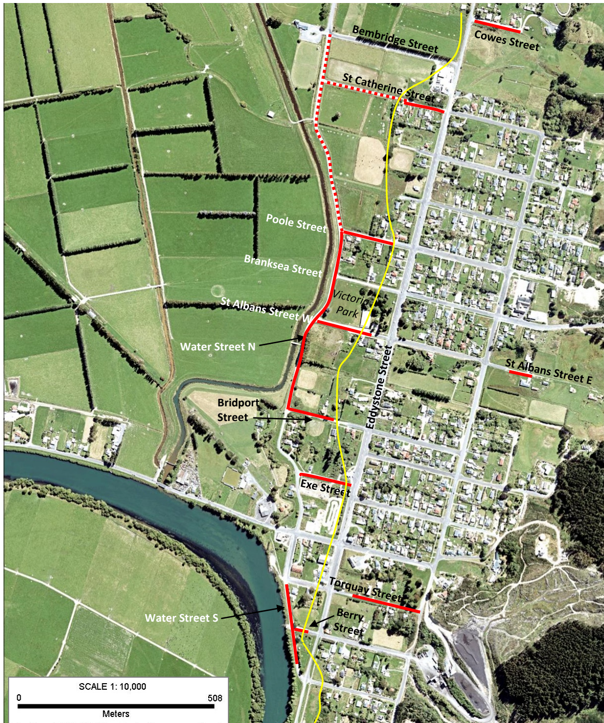
Figure 9. Roads which are currently unsealed in lower Kaitangata. Roads proposed for sealing as part of this project are marked as a solid line. The approximate extent of the flood hazard area is marked as a yellow line.
