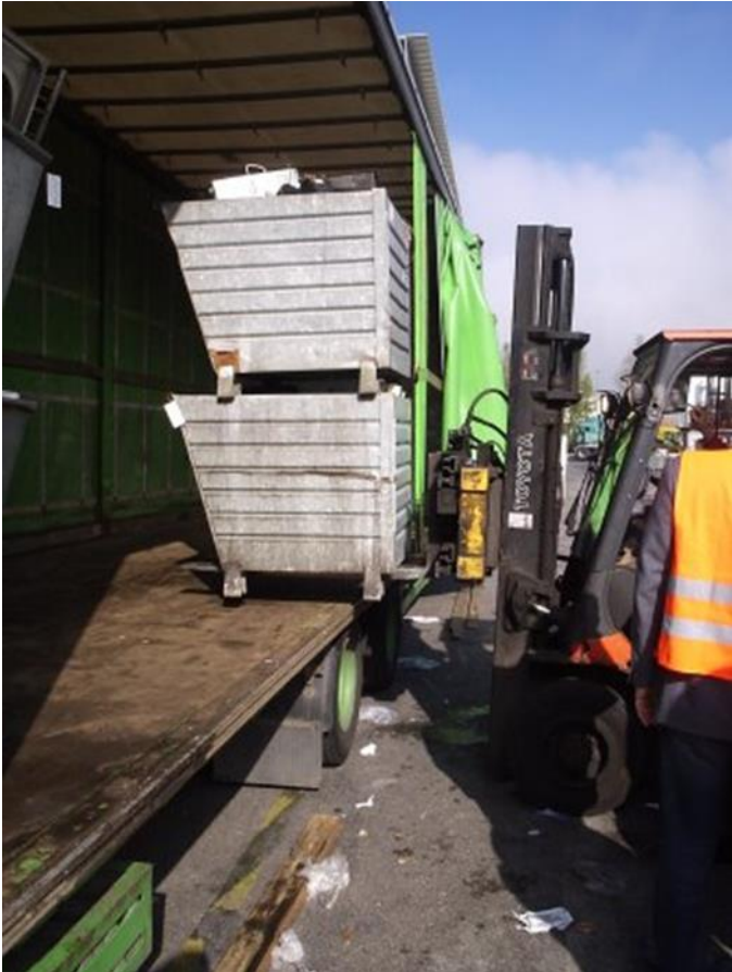
Figure 16: Standardised Bins Being Loaded onto Curtainsider Truck
