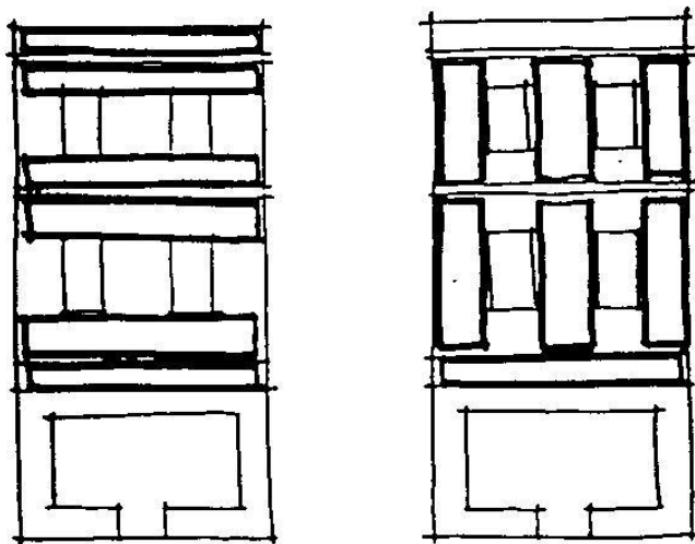
Figure 15 - Horizontal or Vertical Panels
